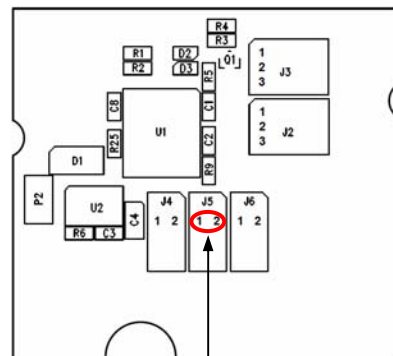
Fig. 4 The jumper circuitry for RS422
