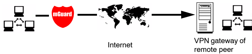
Fig. 6-3 The address of the gateway to the private network where the remote communication partner can be found.
